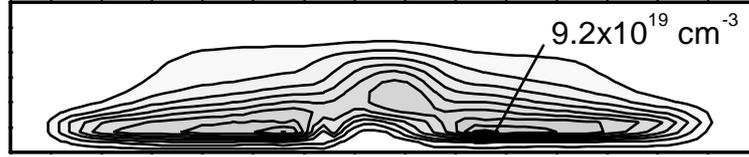
Figure 8.3. Time averaged profile of the effective excitation rate of  $\text{Xe}^* (^3P_1)$ , as calculated with the fluid model. The discharge geometry and conditions are shown in Fig. 8.2; the xenon percentage is 5%. The averaging was done over one address pulse and five sustain pulses. The increment of the contours is  $9.2 \times 10^{18} \text{ cm}^{-3}$ .
